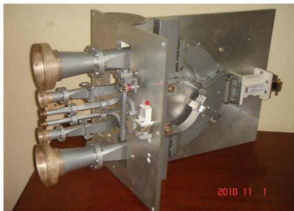
We completed reconstruction and laboratory tests of the three-frequency (of the ranges 4.8, 11.2 and 22 GHz) wideband radiometer «Eridanus» (Fig. 48, left) meant for the monitoring of electro-magnetic interferences in the RATAN-600 operational ranges of (SAO Report 2009, p.80).
